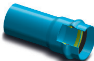
Axonometric view of PVC-A pipe with Forsheda Powerlock gasket mechanically hot pre-inserted during the belling phase of the pipe
