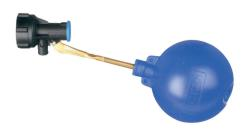
FEATURES & BENEFITS: Working pressure: 0,2÷12 bar ● High performance: 34 l/m at 2 bar - 56 l/m at 5 bar ● Ability to attach a diffuser hose to reduce water turbulence and noise ● UVresistant materials.
